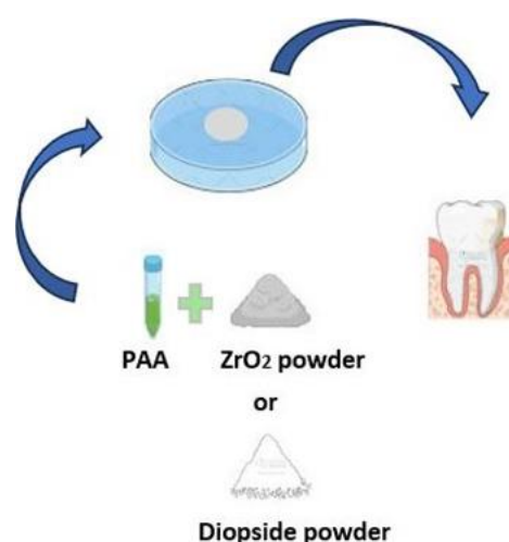
Fig. 1. The schematic illustration of the fabrication method of glass inomer cement
